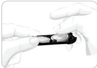
4. Make sure the '+' sign is facing down on the new batteries.
