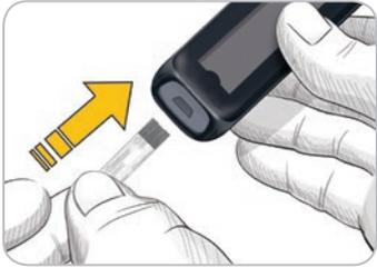
4. Insert the grey square end of the test strip into the test strip port until the meter beeps.
